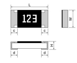
Rated resistance is marked with 3-digit (E24) or 4-digit (E96) on the over coating. RVC16 : only 3digit marking is available.
